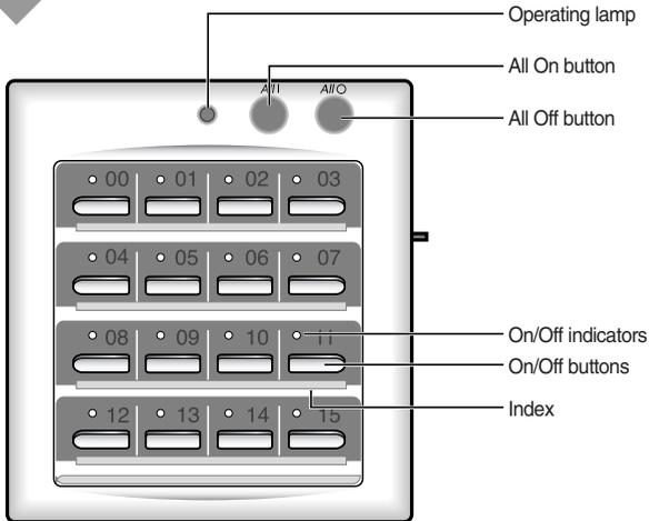
**Note** ◆ The operating lamp comes on even when only one air conditioner connected to the centralized controller is operating.
